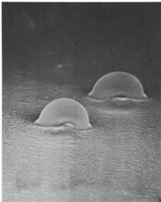
Fig. 2. SEM photograph of the liquid stationary phase (UCON LB-550X). Glass WCOT column, d_c = 250 \mu\text{m} . Magnification 3000 times.
